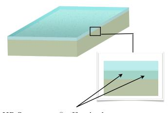
HP Spartacote® effectively absorbing into ("wetting") the substrate.
